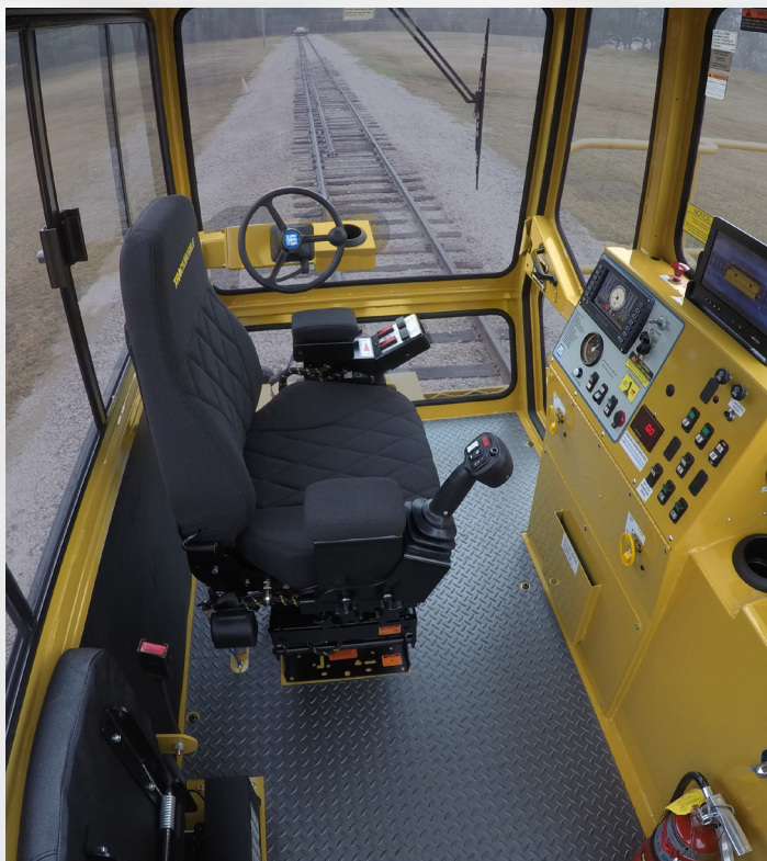
Hercules control panel and operational controls.
